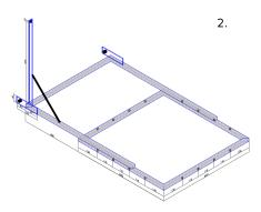
2. Isometric view of the chamber frame. Measures are in mm.
