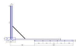
4. Side view of the chamber frame. Measures are in mm.
