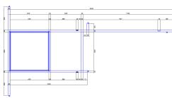
3. Overhead view of the lower frame. Measures are in mm.
