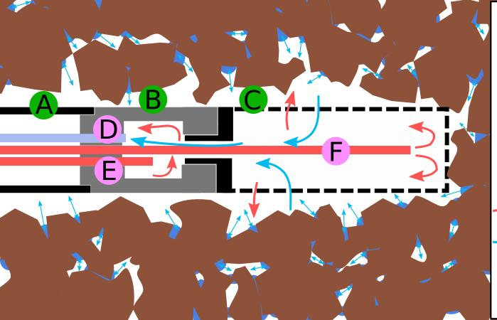
Insertion Shaft Mixing Chamber Microporous Head **D** Sample Line **Dilution Line** F Through-Flow Line Dry Air Flux H<sub>2</sub>O Vapor Flux Soil Water Soil Aggregate
