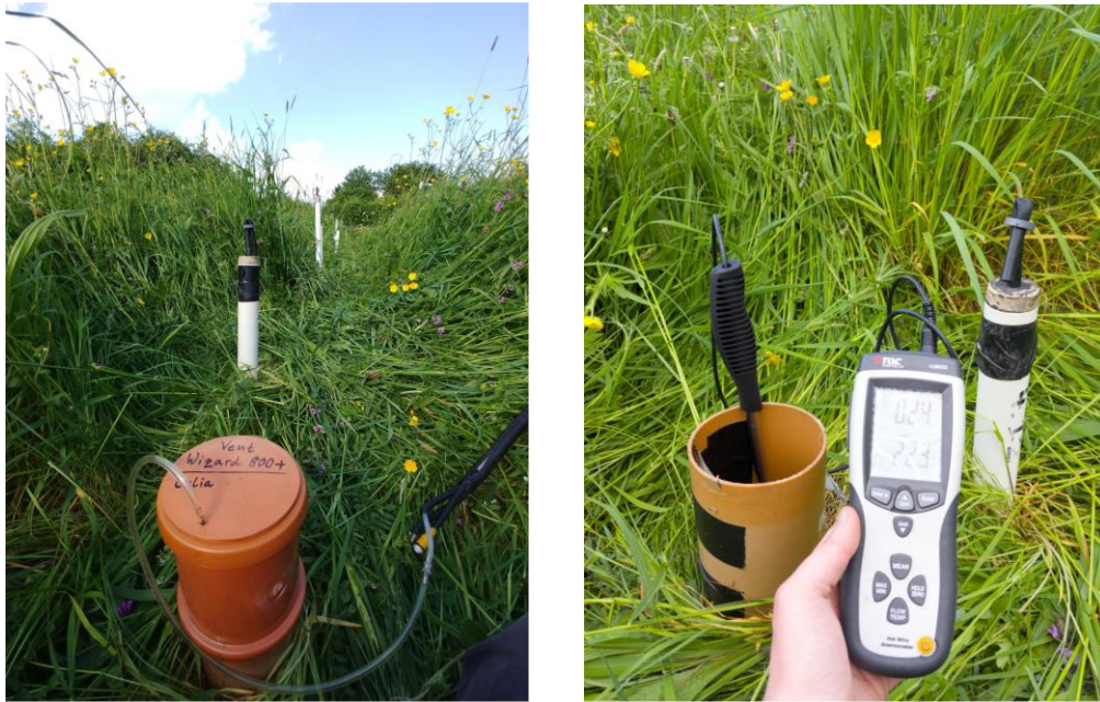
Figure 3. (a) sampling GHG fluxes from the vent system outlet with Vent Wizard 800 (b) deployment of anemometer.
