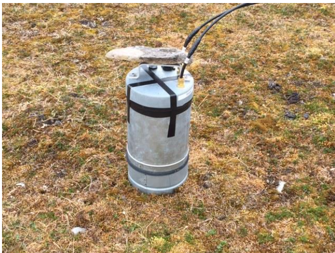
Figure S2. Left: Detail of the soil efflux chamber for CO 2 and CH 4 measurements. Right: Overview of the chamber system with frame, chamber, gas analyser, power supply and laptop.
