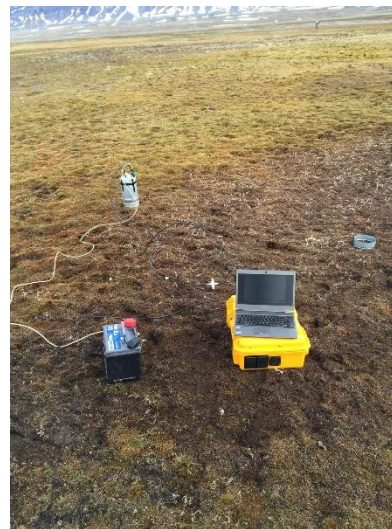
Figure S2. Left: Detail of the soil efflux chamber for CO 2 and CH 4 measurements. Right: Overview of the chamber system with frame, chamber, gas analyser, power supply and laptop.
