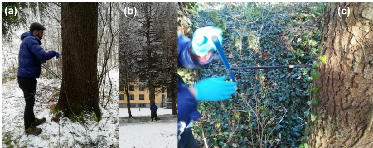
Figure S1.1: Images of sampling (a) Norwegian spruce ( Picea abies ) and (b)(c) European larch ( Larix decidua , left) with an 5.15 mm diameter increment borer.
