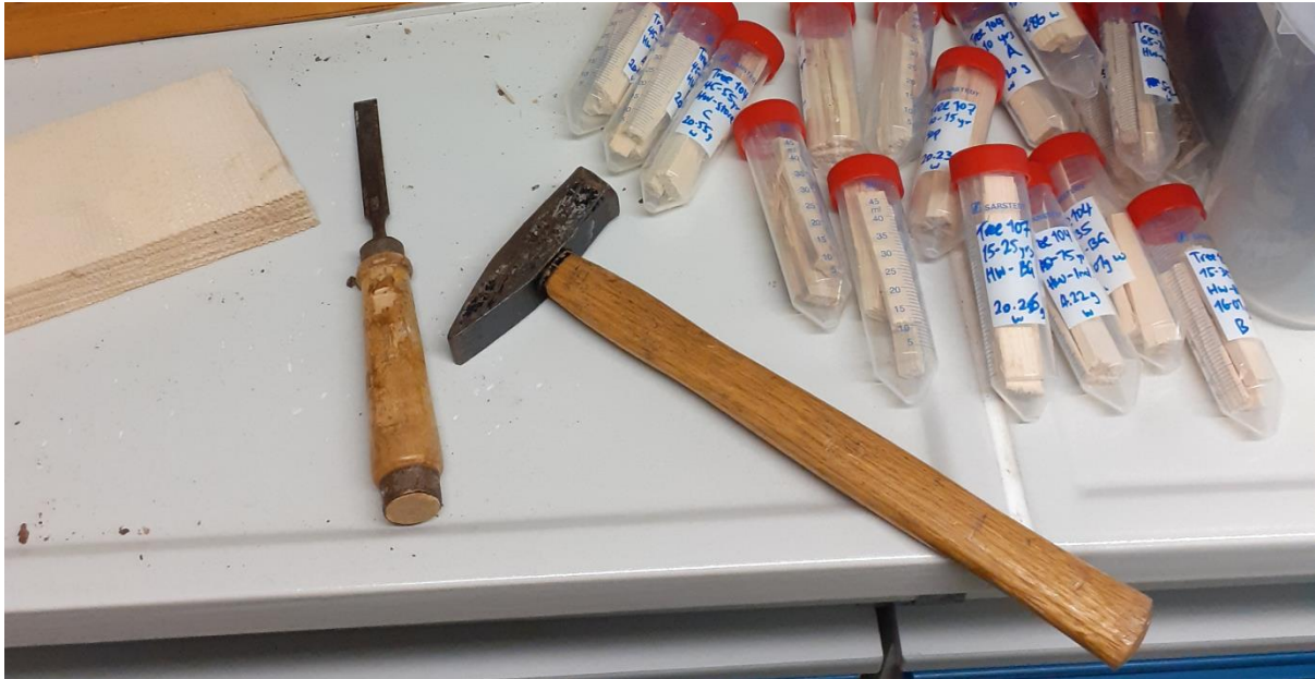
Figure S1.3: Breaking up of samples with chisel for final use. All exposed surfaces after drop saw cut were removed. Chisel and surface was cleaned (see below) between each sample.
