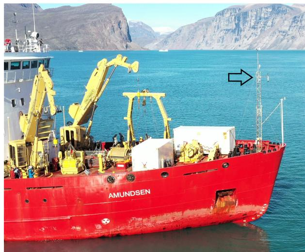
**Figure A1.** The measurement tower at the bow of the ship with anemometer, temperature sensor, and air inlet mounted on the truss approximately where the arrow is pointing. The GPS was fixed at the lower end of the truss. Photo credit to David Cote (DFO – Fisheries and Oceans Canada).
