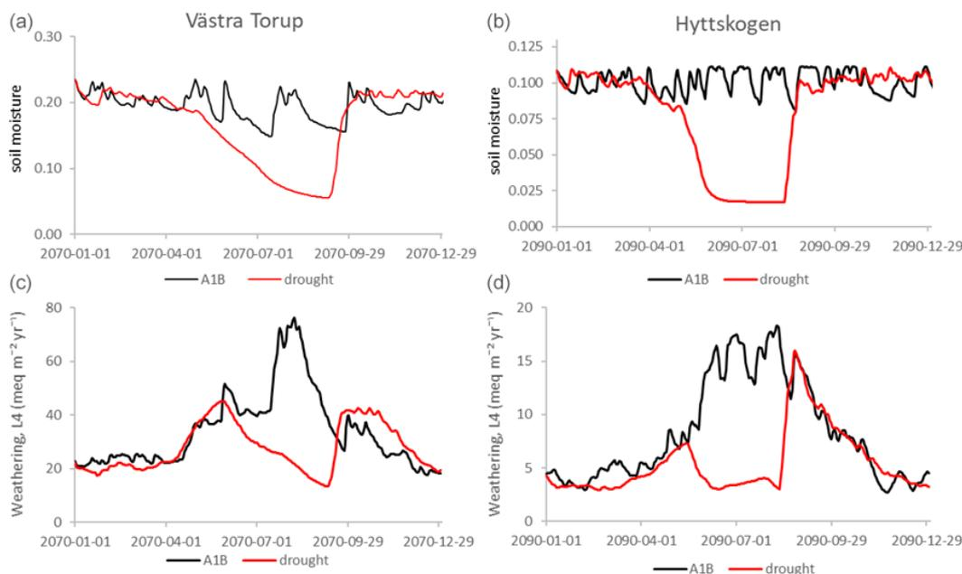
**Figure 6.** Different reactions of soil moisture (a, b) in sites with different texture during the first of the drought years: Västra Torup is less coarse textured than Hyttskogen is and retains water for longer but also infiltrates water slower when precipitation resumes. This also affects the reaction of weathering rates of base cations to droughts (c, d).
