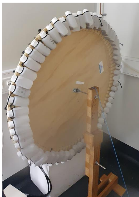
Figure S1. The plankton wheel used for experiments 1, 2, and 3. The picture shows the plankton wheel with incubation bottles mounted on it.
