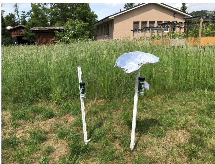
Figure F1. Example of shielding experiment with aluminium foil to determine if the logger measurements were affected by direct sunlight on the thermocouple. The thermocouple on the right pole was placed such that it was shaded throughout the day. The actual experiment consisted of a paired design, where we placed two shielded and two unshielded thermocouples in each of three representative environments for the field sampling (open, trees outside forests, and forest).
