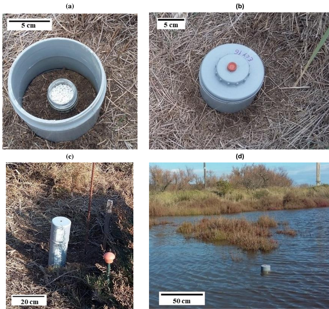
Figure S3. Opaque chambers used to take the measurements of net soil CO 2 and CH 4 fluxes under non-flooded (a, b) and flooded (c, d) conditions. When soil was not flooded, soda lime was placed inside the chamber (a) and then it was hermetically closed (b).
