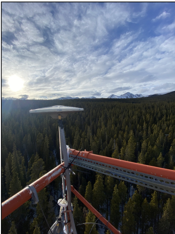
Figure S1. Photos of (a) the gnssA antenna at the top of the US-NR1 26-m tower, and (b) the gnssB antenna mounted on a tripod above the forest floor. The white enclosure shown in (b) , housed the gnssB receiver and the photo is taken northwest of the antenna so that the trees south and southeast of the antenna are shown.
