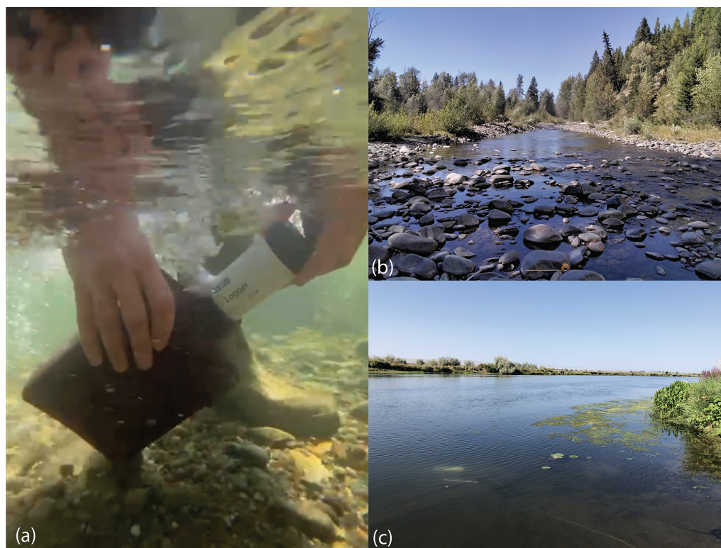
Figure 1. Modified semi- in situ dark bottle incubation method and example study sites. (a) Underwater photograph of DO sensor being inserted into an incubation bottle filled with river water and the mixing device. Panels to the right emphasize the diversity of environmental settings covered in this study. (b) North Fork Teanaway River (site S19E), Kittitas County, Washington, September 2021. Site S19E is classified as a mesic, high-elevation site dominated by tree canopy (cluster 1; see Tables 1 and S3 and Fig. S1). (c) Yakima River at Mabton (site T02), Yakima County, Washington, September 2021. Site T02 is classified as a mesic, middle-elevation site dominated by tree canopy (cluster 5; see Tables 1 and S3 and Fig. S1).
