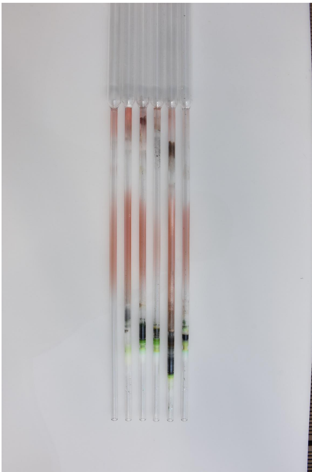
Fig S5: The image of outer quartz tubes indicates significant corrosion and a mass of remnants after analyzing acid-fumigated subsamples. From the left to the right, the first is a recently washed quartz tube; the second has undergone combustion of numerous (>20 counts) acid-rinsed samples; Others are the quartz tubes that have been utilized to analyze acid-fumigated samples in this study (SR1, SR2, Sed1, and Sed2). The black remnants likely result from incomplete combustion, whereas the green parts are likely chlorides.
