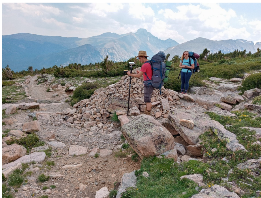
Figure A2. Lucas Rudasill and Laurel Sindewald collecting a ground control point and descriptive metadata at the corner of a switchback next to a cairn in RMNP. This photo was included, with the GPS data, descriptive metadata, and image chips, to inform MAXAR orthorectification.
