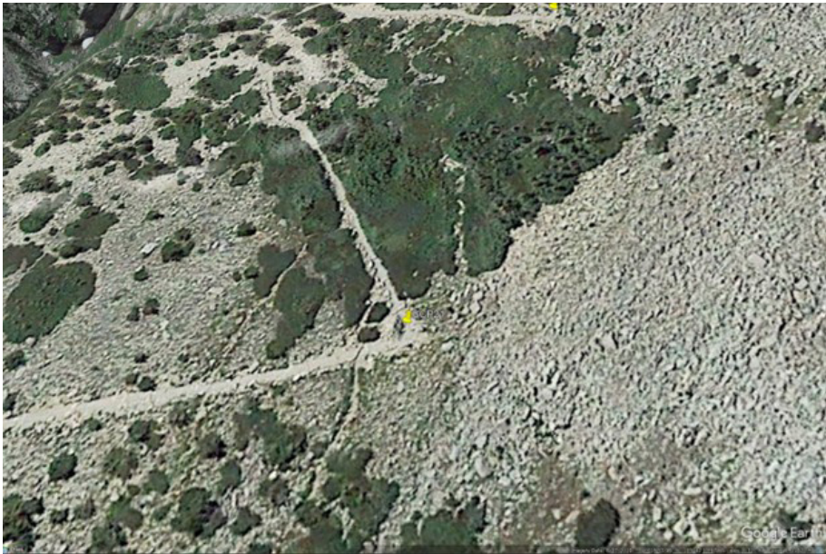
Figure A3. Example of an image chip from Google Earth Pro with the GCP position marked precisely on the image, corresponding to the photo documentation in Fig. 26. This image chip was included, with the GPS data, descriptive metadata, and photos, to inform MAXAR orthorectification. © Google Earth.
