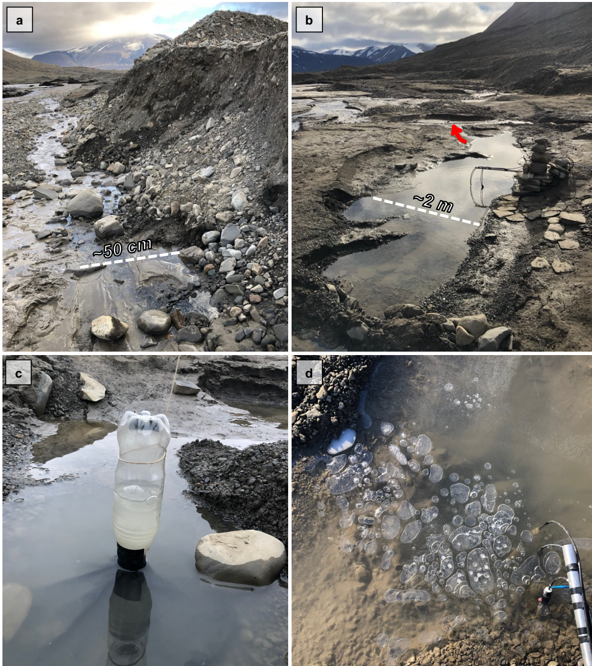
Figure S.2. (a) GW1 spring outflow, with outlet stream flowing towards the top left corner of the picture, (b) GW2 pool—pool formed over the inflow of the spring with outlet stream marked with red arrow, (c) The bubble trap used to make ebullition measurements, and (d) bubbles resulting from ebullition trapped beneath a thin layer of ice formed on the surface of the GW2 pool during a period with below-freezing temperatures at the end of the summer.
