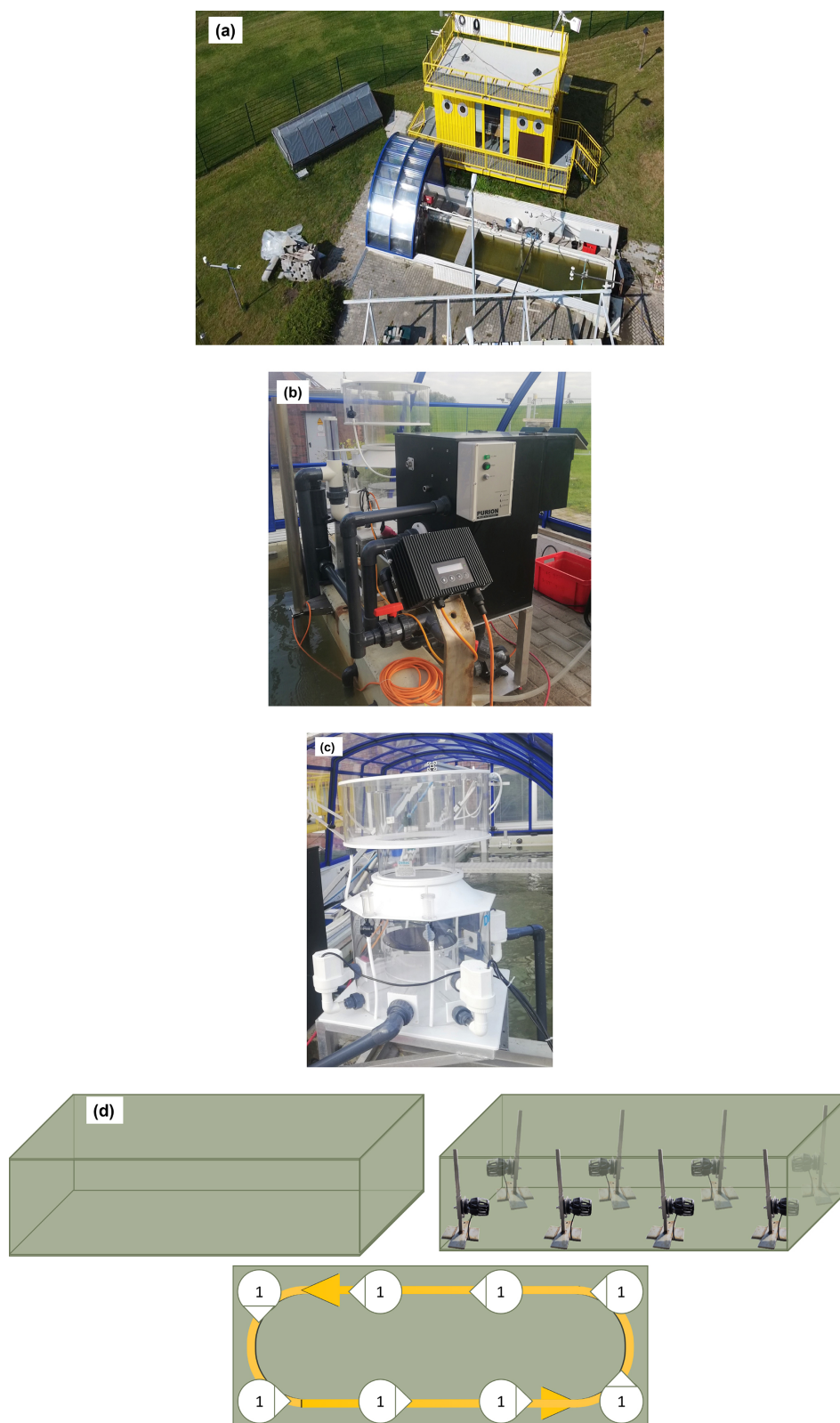
Figure 1. (a) Sea-sURface Facility (SURF) used for the mesocosm experiment. (b) Filtration unit with a fleece filter in the front black box. (c) The Protein skimmer. (d) The top-left panel shows the SURF basin without the pump installed. The top-right panel illustrates the schematic arrangement of eight flow pumps, and the bottom panel shows the direction of the water flow pattern induced by the pumps, ensuring uniform mixing across the basin.
