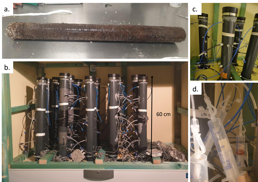
Figure S4. Incubation setup of the mesocosms. Picture of the core from the fen after removing the oven pipe (a.); Incubation chamber with the 15 mesocosms. Here, only the first 60cm were thawed and incubated at 10°C. The bottom part represents the freezer (b.); Zoom in on the mesocosm tubes and the different probes: the 3-way valves, the rhizons and the temperature sensors. The blue cables are connected to the mesocosm headspace and to the Picarro (c.); Water sampling with syringes connected to the rhizons (d.).
