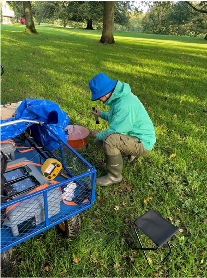
80 Figure S1: Soil greenhouse gases fluxes measurement with the fast closed chamber approach
