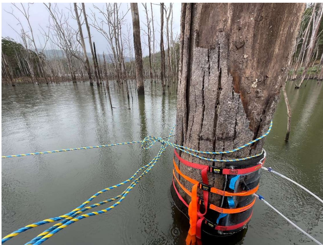
Figure S1: Flux chamber attached against a ghost forest tree at Hinze dam at the lowest measurement on top of Bark.
