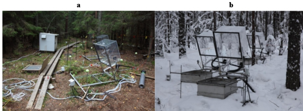
Fig. 1. Photographs of the chamber system in (a) summer position at the Lettosuo site and (b) winter position with additional collars installed at the Kalevansuo site. The frame is lifted by bolts on the five threaded rod legs. Insulation of the cables and tubing is visible in the winter position. Original direction of motors is visible in the summer position, adjusted direction in the winter position.
