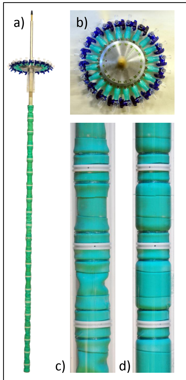
Fig. S4: Pictures of the MLS. a). Full-length picture. b) Top-down picture showing the 20 sampling valves. c) Close-up picture with c) deflated and d) inflated packer membranes in a transparent tube.
