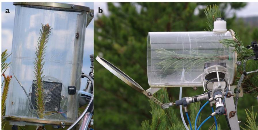
**Fig. 1.** Emission measurements with dynamic shoot enclosures. **(a)** The enclosure with a developing Scots pine shoot in the end of May, when the intensive needle elongation period begins. **(b)** The enclosure with a mature Scots pine shoot.
