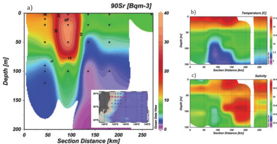
**Fig. 4.** Specific activities of  $^{90}\text{Sr}$  (expressed in Bqm $^{-3}$ ) and temperature and salinity contour plots in a section at Fukushima NPP latitude. It comprises stations 25 (left hand, closest to Fukushima), 23, 21, 19 and 11 (right hand).
