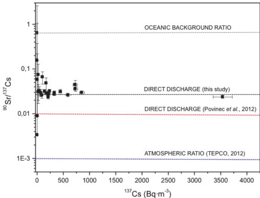
**Fig. 8.** The  $^{90}\text{Sr}/^{137}\text{Cs}$  ratio as a function of  $^{137}\text{Cs}$  specific activities. The grey dashed line represents the oceanic background ratio decay corrected to 2011. Also shown are the  $^{90}\text{Sr}/^{137}\text{Cs}$  ratios corresponding to the oceanic background ratio, the direct discharges from Fukushima Dai-ichi and the atmospheric deposition.
