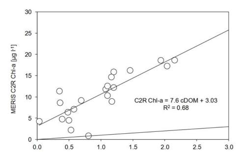
**Fig. 7.** TRANSDRIFT-XVII acDOM440 (from 9 to 20 September 2010) vs. MERIS C2R\_Chl a calculated from the MERIS acquisition on 7 September 2010, n = 23.
