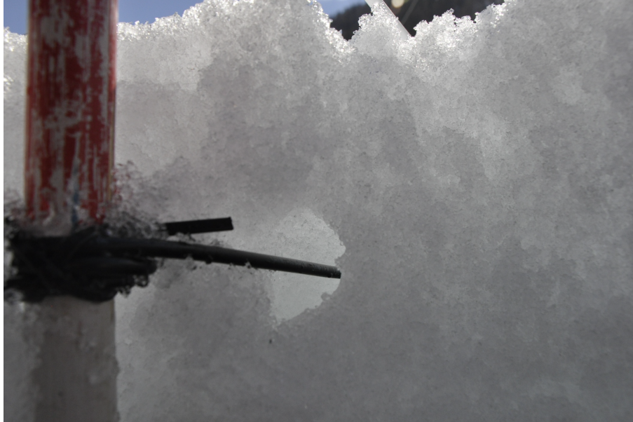
Fig. 6. Ice channels, which developed over the course of the season around the tubing of the automatic gradient measurement system. Therefore \text{CO}_2 and ^{222}\text{Rn} measurements incorrect (photocredit L. Merbold).
