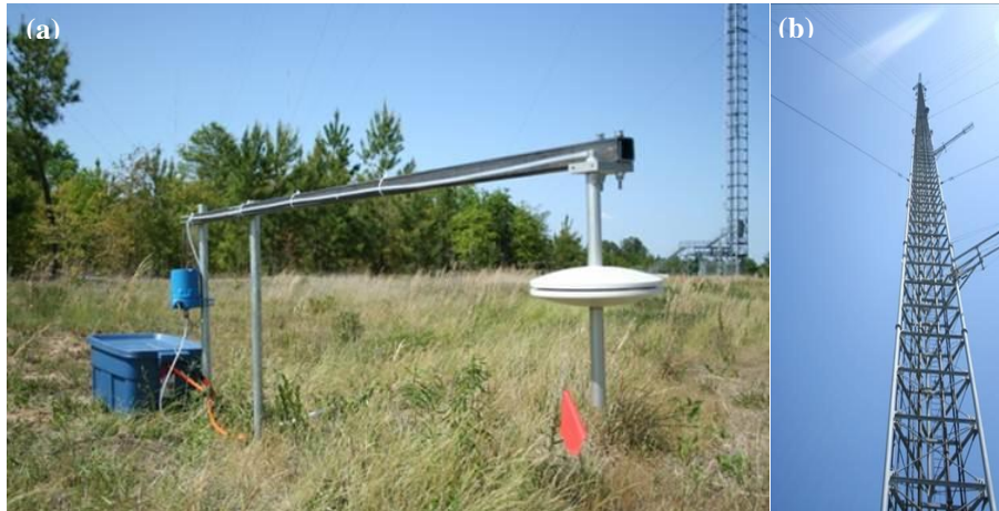
Fig. 1. (a) A microbarograph station and (b) the tall tower with flux measurement levels at 34, 68, and 329 m
