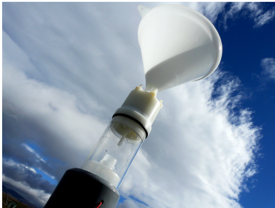
Fig. 2. Rainwater sampling device on the top of its PVC tube.
