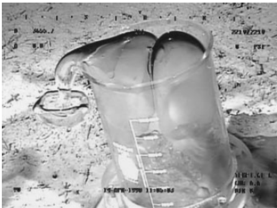
Fig. 8. From Brewer et al. (1999). An experiment in deep ocean fossil fuel CO 2 disposal. A 4 L laboratory beaker was placed on the sea floor at 3650 m depth and about 2 L of liquid CO 2 dispensed into it to observe hydrate formation effects and test theory. A CO 2 hydrate “ice storm” occurred at the interface and slush of solids accumulated at the bottom, pushing excess liquid out of the top. A large fish and other deep-sea animals came by. This image captured significant attention and also aroused latent concerns.
