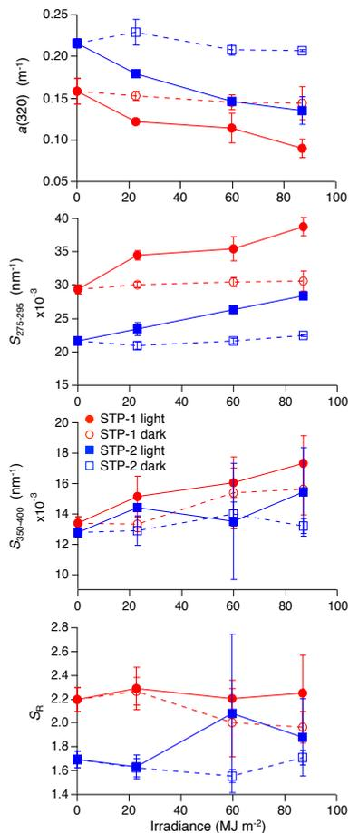
**Fig. 6.** Changes in  $a(320)$ ,  $S_{275-295}$ ,  $S_{350-400}$ , and  $S_R$  during photo-irradiation experiments of the subtropical deep waters. Note: 23, 60, and 87 MJ m<sup>-2</sup> on the X-axis was corresponding to 2, 6, and 13 days for the dark control experiments, respectively.
