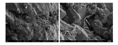
**Fig. 1.** Secondary electron images of the calcite rhombs in the cavities. Arrow indicates a microbial filament, which is associated with these rhombs.
