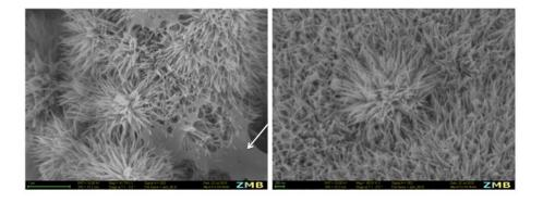
**Fig. 2.** High-magnification secondary electron images of the rosette structures, which are composed of acicular nano-fibers. The image on the left also shows EPS (see arrow).
