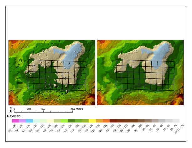
**Figure S1**: LVIS ground correction. Raw LVIS ground returns (left) and corrected LVIS ground returns (right) using the DRL Digital Elevation Model.
