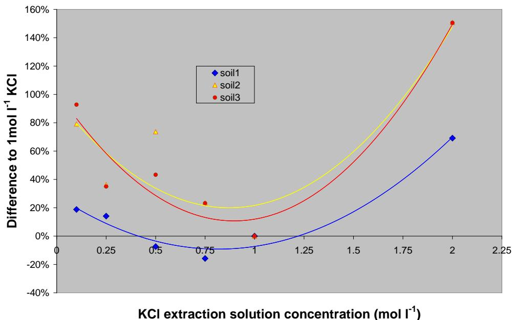
Fig. 1. Influence of the KCl extraction solution concentration (range 0.1 to 2 M) on the soil NH<sub>4</sub><sup>+</sup> extraction efficiency. The results are expressed as the percentage difference in extracted NH<sub>4</sub><sup>+</sup> relative to the 1M KCl extraction, which was the authors standard procedure.
