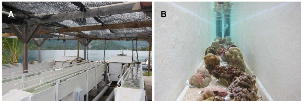
**Figure 1.** Photographs of the outdoor flumes. **(A)** The flumes consisted of a 5.00 m × 0.30 m × 0.30 m working section, and a lower sediment chamber (2.50 × 0.30 × 0.25 m) in which sediments were maintained, and together contained ~ 600 L of seawater. **(B)** Communities matching the average composition (in 2013) of the back reef in Moorea were constructed in the flumes.
