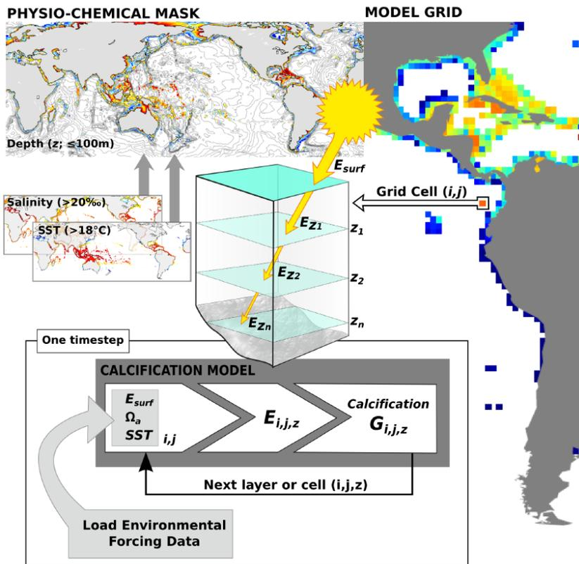
**Figure 2.** Schematic of logical steps at each timestep within GRAM. GRAM's domain is defined by a bathymetric and physiochemical mask within which calcification is calculated, at each timestep and in every domain grid cell, according to the calcification model used. Where calcification is modeled as a function of light, the availability of light at depth ( $E_z$ ) is calculated for each model layer ( $z_i$ ).
