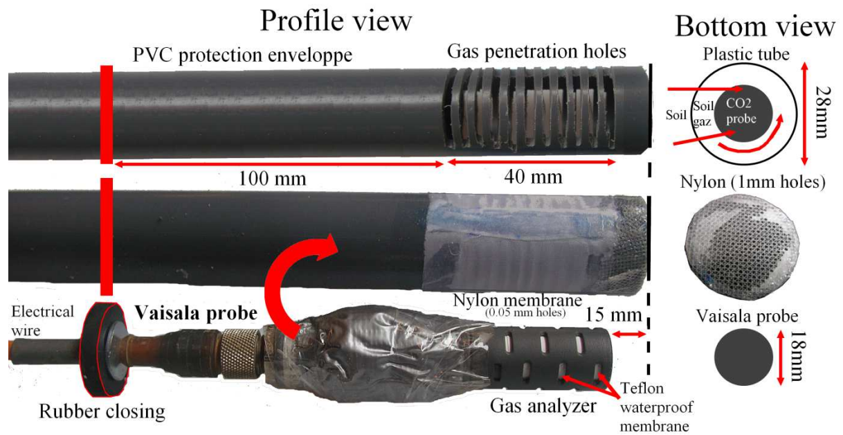
Fig. 3. Description of the probes used for CO 2 concentration measurements inside the soil.
