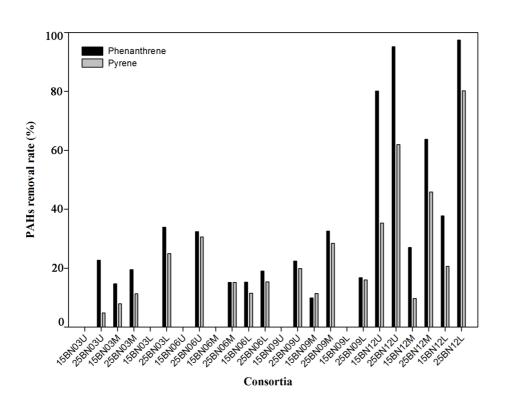
**Figure 4.** PAH-removal rates of the consortia that were enriched from the sediments of the Arctic Ocean. The consortia were grown with a mixture of PAHs (naphthalene, phenanthrene, and pyrene) as the sole carbon and energy source. PAHs were quantified using GC/MS after pretreatments. Naphthalene was not included due to an error caused by its apt volatility. Consortia names with prefixes "15" or "25" indicated they were enriched at 15 or 25 °C, respectively.
