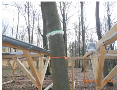
Figure 3. Roof construction sketch of the main roof (10 m × 10 m) (a) . Roof with panels, rain gutters and water barrel and main tree (b, c) . Roof detail with main tree and stem rim to collect stem flow (d) . All pictures were taken at plot SEW48.
