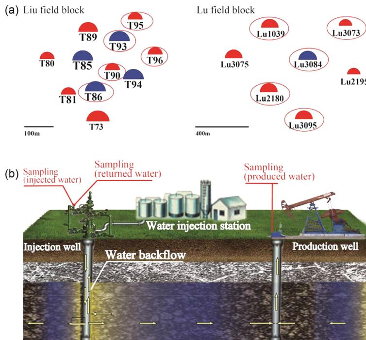
**Figure 1.** The schematic diagram revealing (a) the distribution of the injection and production wells of Liu and Lu field block, and (b) the wellhead and downhole of injection wells and production wells, and the place where water samples were collected. The selected T86, T93 and Lu3084 are injection wells, while the selected T90, T95, T96, Lu1039, Lu2180, Lu3073 and Lu3095 are production wells.
