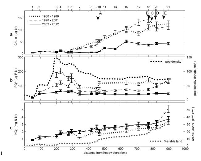
Figure 2. Longitudinal profiles of summer median Chl. a (a), winter median PO<sub>4</sub><sup>3-</sup> (b) and  $NO_3^-$  (c). Averages for three periods, in relation to % arable land (2006) and population density (2008) tested as eutrophication control variables. Uncertainty bars are due to sampling frequency. Arrows and capital letters (A to E) represent confluences with major tributaries (Fig. 1).
