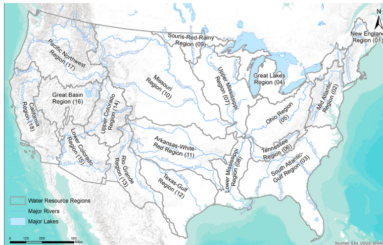
Fig. 1. CONUS water resource regions. USGS water resource regions and major rivers in the CONUS domain. Prior to aggregation of product runoff, regions coverage converted from polygon ( http://water.usgs.gov/GIS/huc.html ) to 1^\circ raster using the region with the maximum area of overlap for each grid cell.
