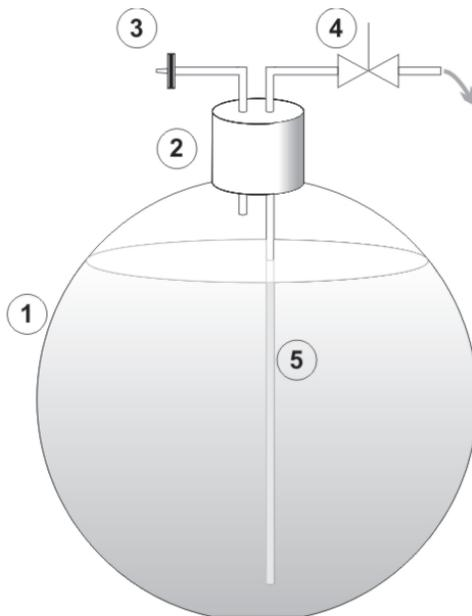
**Fig. 1.** Experimental setup: 11 glass bottles (1, total volume 49 L) each of which contained sterile artificial seawater medium (including additional nutrients), 1 L seawater inoculum and three different substrates. The bottles were closed with a rubber lid (2) and air exchange was enabled by a sterile 0.2 µm filter (3). Samples were taken through a valve (4) using a peristaltic pump and glass (5) and Teflon tubing.
