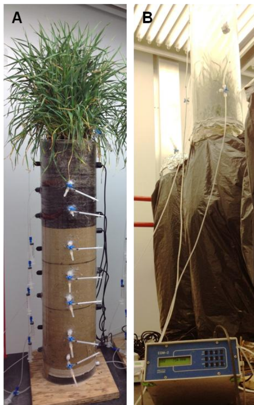
Fig. 1. Mesocosm system with barley plants and sampling ports for gas and water sample collection, soil moisture and temperature measurement (A) and setup for CO 2 exchange measurements (B) . During experiments, mesocosms were shaded from light with dark plastic bags (B) .
