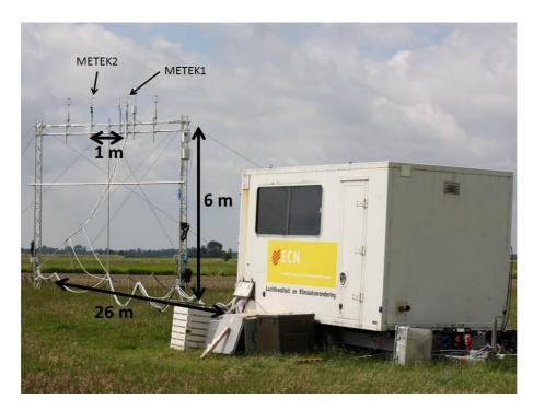
**Fig. 1.** Picture of the measurement setup. The picture was taken towards the most common wind direction during the campaign. The trailer which housed the closed-path instruments and data logging computer is at the front of the picture.
