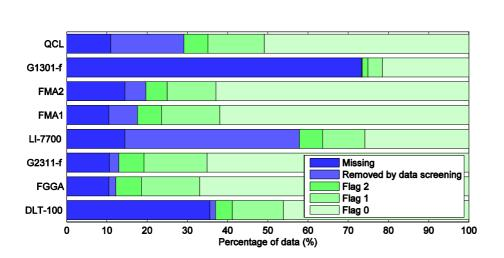
**Fig. 3.** Distribution of quality flags for methane fluxes during the campaign. Quality flags were given according flux stationarity criteria (Foken and Wichura, 1996). Flag 0 (flux stationarity below 0.3) corresponds to highest quality, flag 1 (flux stationarity between 0.3 and 1) to mediocre quality and flag 2 to lowest quality (flux stationarity above 1). Green bars show the amount of accepted data and blue bars shown the amount of omitted data.
