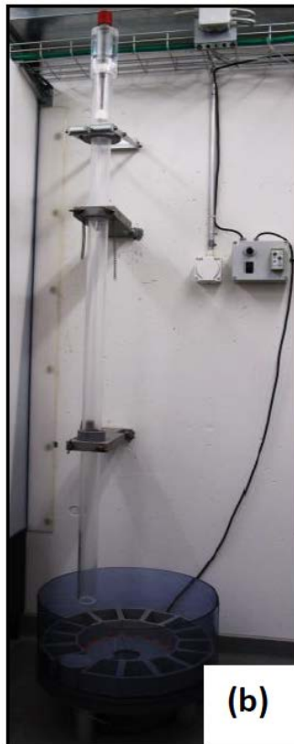
Figure 1. The rainfall simulation flume (a), and the settling tube apparatus (b). The settling tube apparatus consists of four components: the settling tube, through which the soil sample settles; the injection device, by which the soil sample is introduced into the tube; the turntable, within which the fractionated subsamples are collected; and the control panel, which allows an operator to control the rotational speed and rest intervals of the turntable (operations see Hu et al., 2013b).
