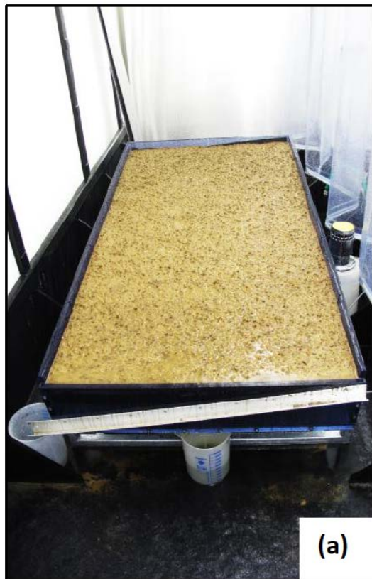
Figure 1. The rainfall simulation flume (a), and the settling tube apparatus (b). The settling tube apparatus consists of four components: the settling tube, through which the soil sample settles; the injection device, by which the soil sample is introduced into the tube; the turntable, within which the fractionated subsamples are collected; and the control panel, which allows an operator to control the rotational speed and rest intervals of the turntable (operations see Hu et al., 2013b).
