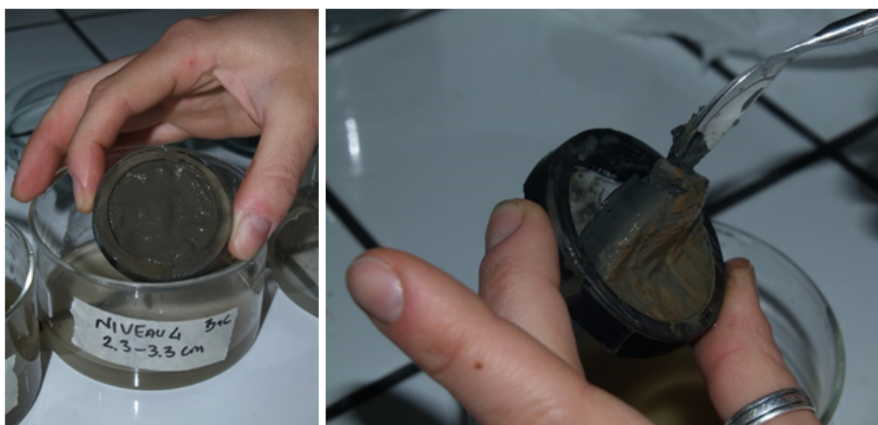
Fig.1 (left) 2.3-3.3 cm deep layer of experiment 2 showing homogeneous light grey color; (right) 0.3-1.3 cm deep layer of experiment 2 showing brownish surface (low oxygen concentrations still present) and grey to dark grey bottom, suggesting that no lateral oxygen penetration occurred at the bottom layer.
