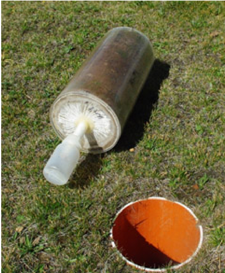
Fig. 1. Micro-Lysimeter installed at Kema site (Photo by S. Willinghöfer, 2012)
