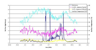
Fig. 8. Sensitivity test. In dark blue: reference NO flux in  $kg(N)ha^{-1}yr^{-1}$ , in yellow: NO flux with H=2% and mineral N=0.01g m<sup>-2</sup>, in pink: NO flux with H=10% and mineral N=0.1g m<sup>-2</sup>, in light blue: surface temperature in °C, for year 2006.
