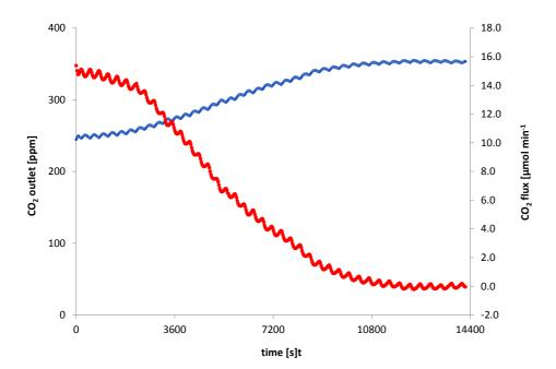
**Fig. 3.** Figure 3: Evaluation of the response time of the chamber system. The Co2 outlet concentration on the left axis is shown in blue, the CO2 flux is shown in red. Steady state is reached after 11800s. The
