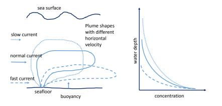
**Fig. 1.** Sketch of a methane plume with a constant source and buoyancy, but different water velocities. The shape of the vertical methane concentration profile would not change.
