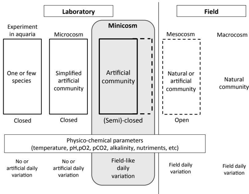
**Figure 1.** Different systems used in OA studies (as discussed in the text). The minicosm (in grey) serves as a compromise between more realism and complexity on the one hand, and ease of maintenance and replication in the laboratory, in the other hand.
